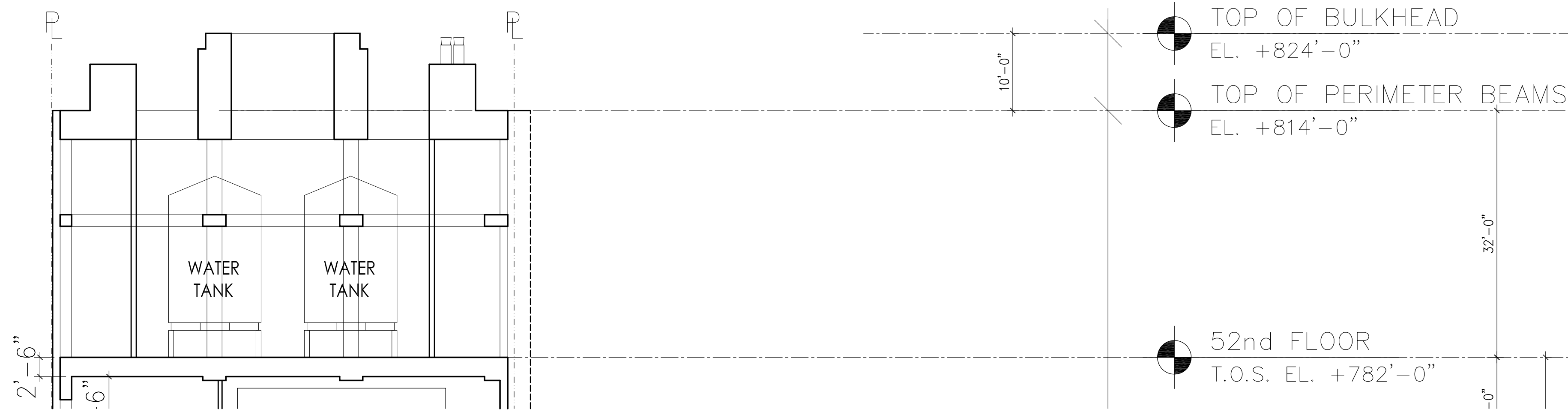
02 PARTIAL SECTION - MECHANICAL TERRACE OPEN TO THE SKY SCALE: 3/32" = 1'-0"
